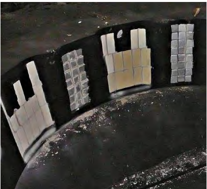
IZOCAST blocks during moulding. Casting for the shipping industry.
