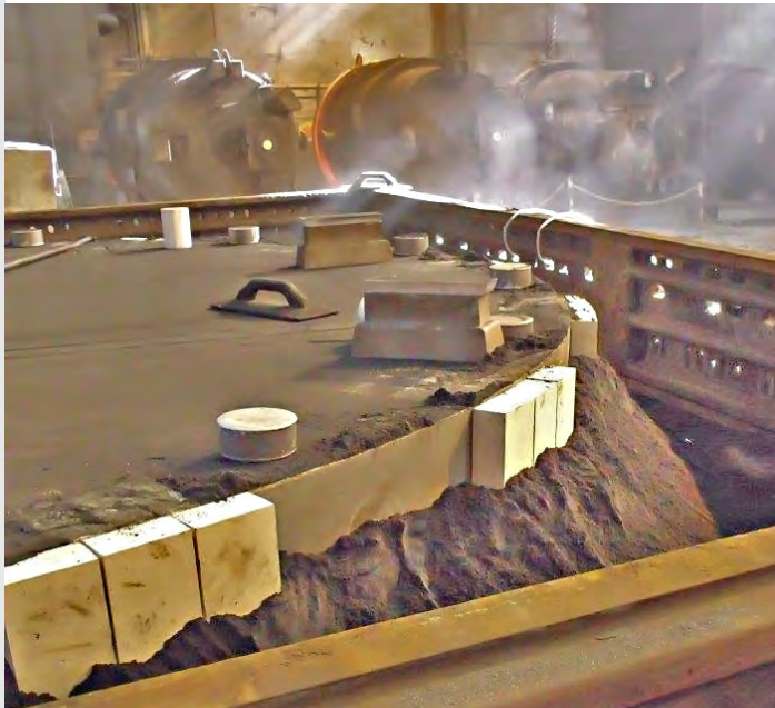
Example of use of the IZOCAST blocks in a foundry: moulding the Francis turbine rotor rim.
