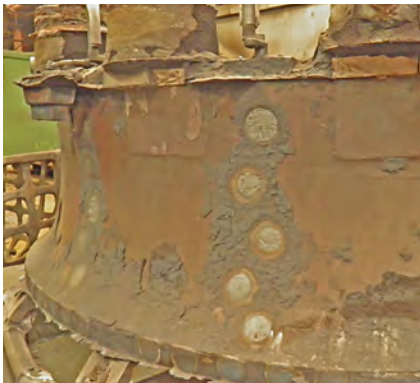
Unit after casting and demoulding, on which the IZOCAST blocks were used in certain zones.
